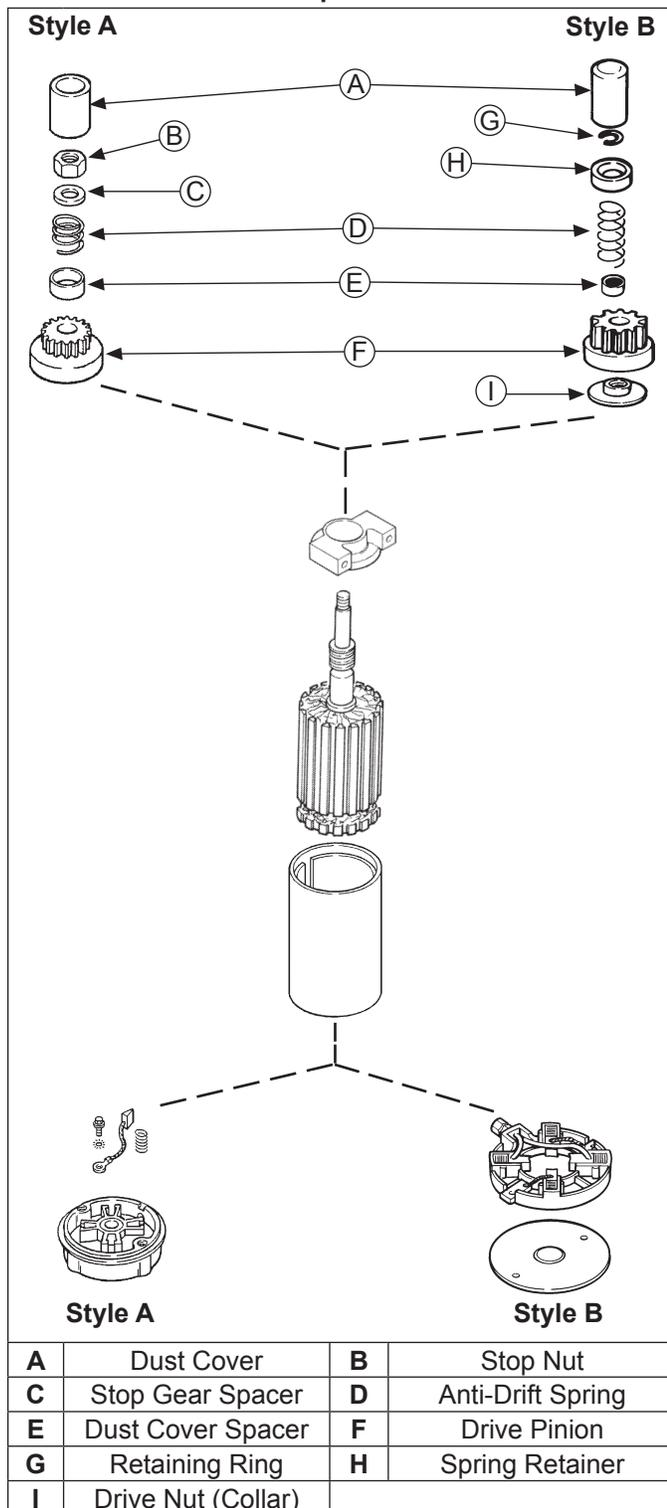
When power is applied to starter, armature rotates. As armature rotates, drive pinion moves out on drive shaft splines and into mesh with flywheel ring gear. When pinion reaches end of drive shaft, it rotates flywheel and cranks engine.
