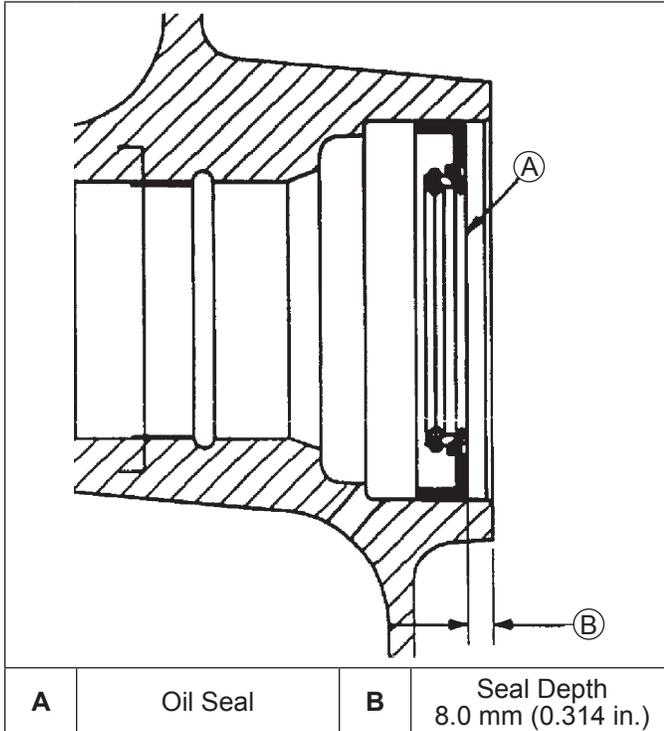
1. Check to make sure there are no nicks or burrs in crankshaft bore of closure plate.
