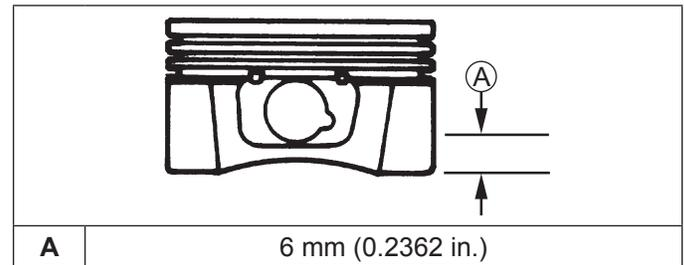
**NOTE:** Do not use a feeler gauge to measure piston-to-bore clearance—it will yield inaccurate measurements. Always use a micrometer.
