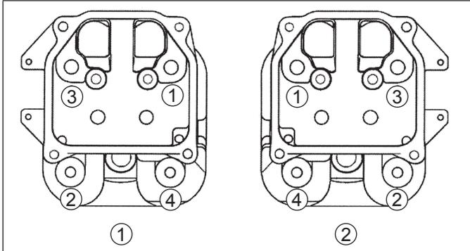
**NOTE:** Cylinder heads must be attached with original type of mounting hardware, using either screws, or mounting studs with nuts and washers. Heads are machined differently for studs than for screws, so fastening method cannot be altered unless heads are being replaced. Do not intermix components.
