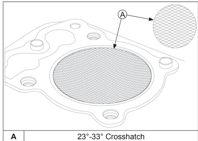
**NOTE:** Some CH25 engines feature POWER-BORE™ cylinders a special patented nickel-silicone plating process for increased power, superior oil control, reduced exhaust emission, and virtually permanent cylinder life. POWER-BORE™ cylinders cannot be resized or honed as described in these procedures. If a plated cylinder bore is damaged or out of specification, use a new miniblock or short block to repair engine. Use following procedure for crankcases with a cast iron sleeve.
