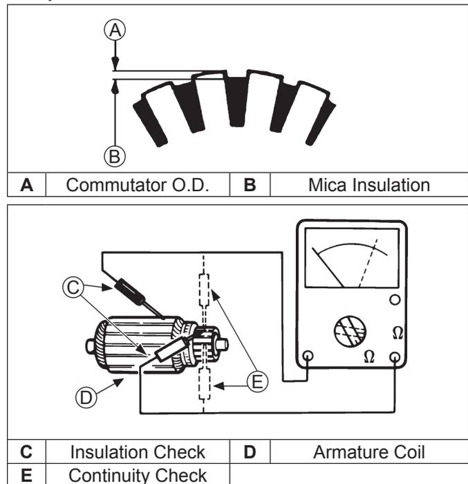
1. Clean and inspect commutator (outer surface). Mica insulation must be lower than commutator bars (undercut) to ensure proper operation of commutator.
