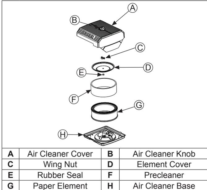
**NOTE:** Operating engine with loose or damaged air cleaner components could cause premature wear and failure. Replace all bent or damaged components.
