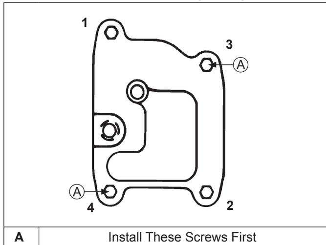
RTV sealant was used on early models between breather cover and crankcase. A gasket with imprinted sealant beads is now used and recommended. Install as follows:
