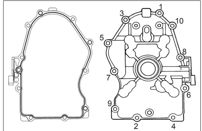
RTV sealant is used as a gasket between closure plate and crankcase. Always use fresh sealant. Using outdated sealant can result in leakage.
