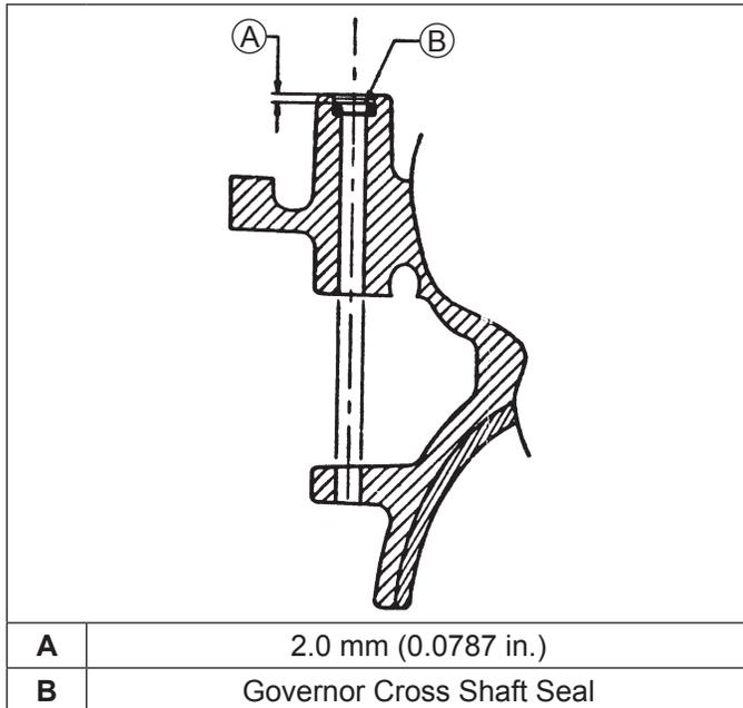
If governor cross shaft seal is damaged and/or leaks, replace it using following procedure.
